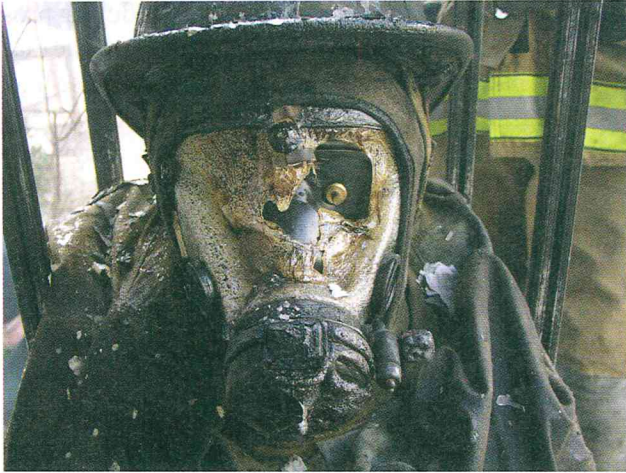
FIGURE 15-8 Thermal degradation of an SCBA facepiece.
