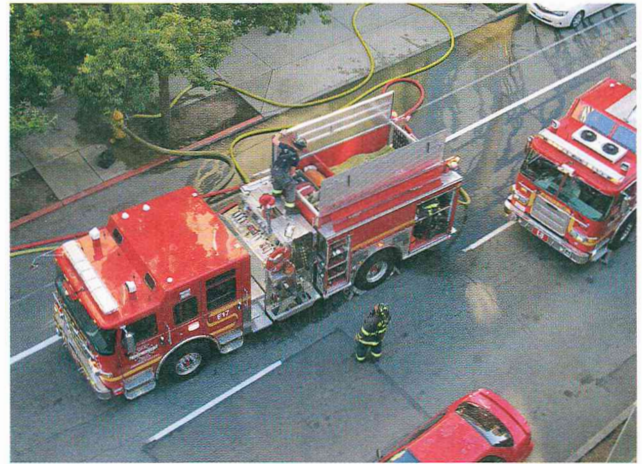
FIGURE 15-13 Positioning the first-in pumper within 100 feet of the hydrant and 100 feet of the standpipe FDC reduces friction loss.
