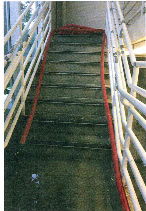
FIGURE 15-43 The RIT line can be connected on the fire floor hose outlet and coiled on the stairway landing above the fire floor. The combination nozzle can be left unattended in a state of readiness. The door to the fire floor should be closed as tightly as possible.
