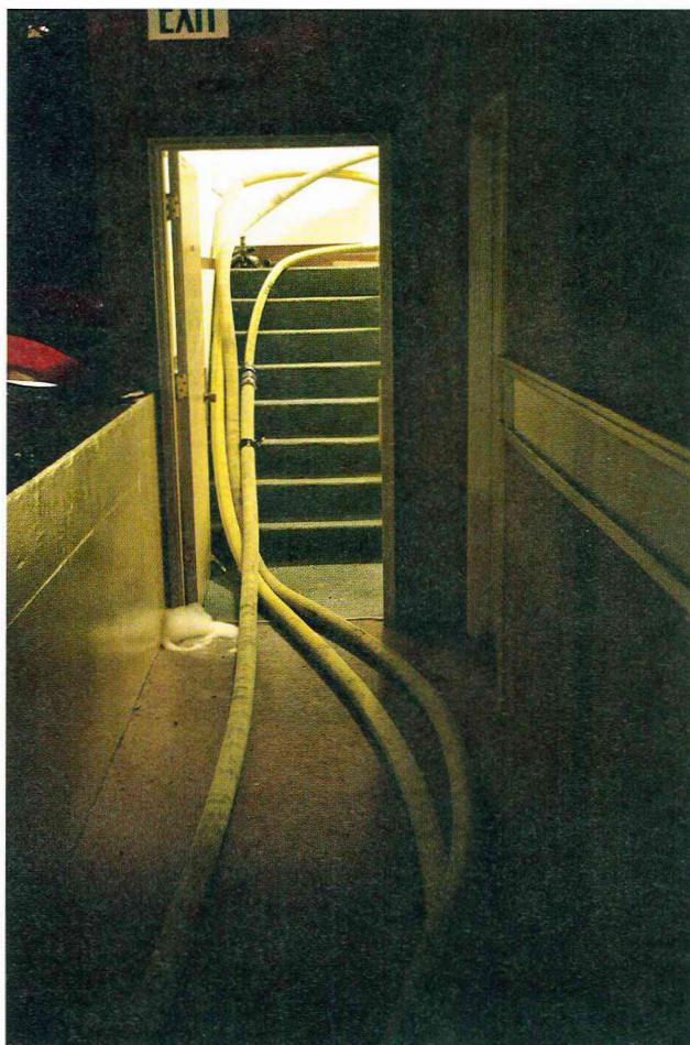
FIGURE 15-40 Three charged 2½-inch lines in a single stairwell are unmanageable.
