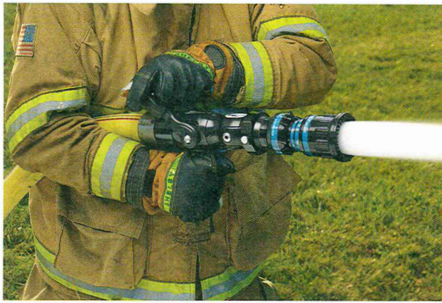
FIGURE 15-22 TFT Flip-Tip nozzle: A. the combination fog nozzle and B. the smooth-bore tip.
