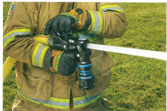
FIGURE 15-22 TFT Flip-Tip nozzle: A. the combination fog nozzle and B. the smooth-bore tip.
