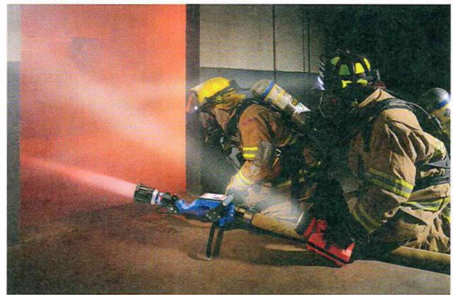
FIGURE 15-23 The lightweight, single-operator TFT Blitzfire portable monitor.
