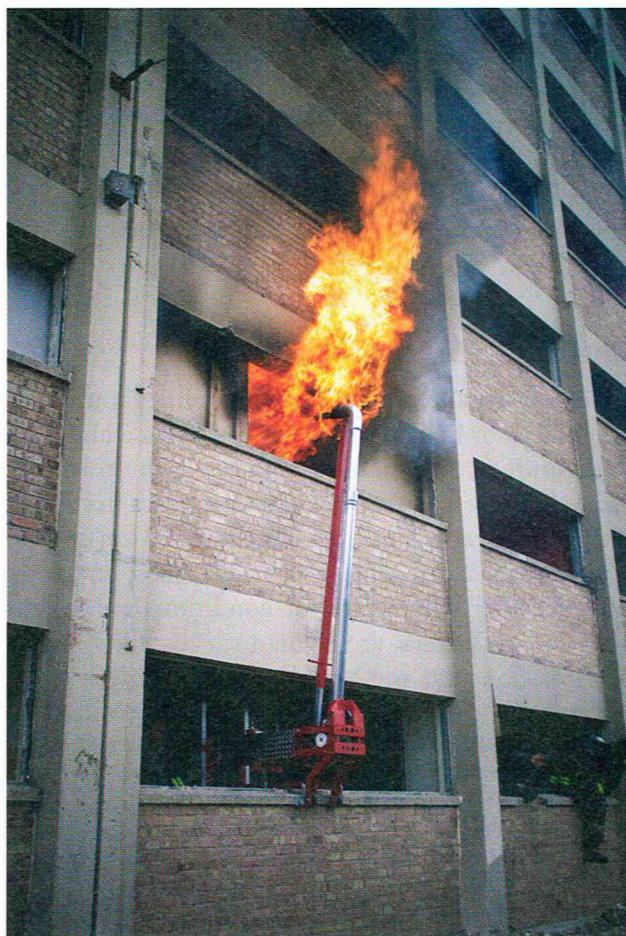
FIGURE 15-50 With a 1½-inch or 1⅞-inch smooth-bore tip, the HEROPipe can flow up to 900 gpm.
